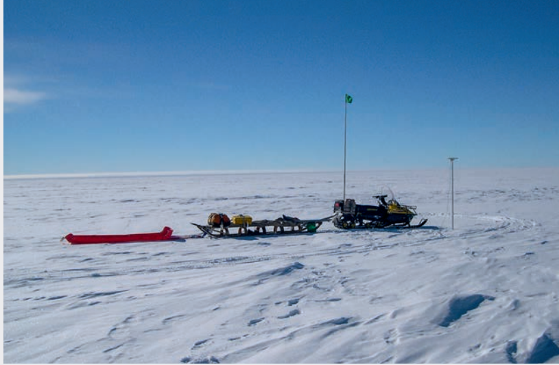
Top: A GPS antenna and associated equipment on the Whillans Ice Stream in Antarctica in 2015, placed to help scientists better understand how fast the ice is moving.
